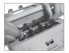
2 Raise the two plastic "T" handles at the same time and hook them onto the metal shaft.
