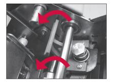
5 Unhook the two plastic "T" handles from the metal shaft and lower them at the same time.
