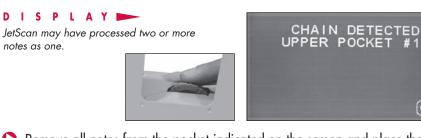
Remove all notes from the pocket indicated on the screen and place them on the hopper. Press CONT. If the alarm repeatedly occurs, adjust the gray thickness adjustment dial located on top of the machine behind the hopper extension. Rotate in the negative (-) direction as indicated by numbers on front of the dial.
