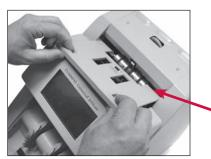
Replace feeder plate. Insert curved edge of feeder plate first. Gently press down on feeder plate until it snaps into position.
