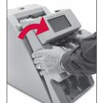
**6** Firmly push down on left and right release levers and pull front enclosure open for access to paper path.
