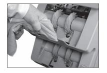
12 In pockets one and two, use a microfiber towel or vacuum to clean the stacker mirror located directly across from the stacker-sensor lens.
