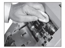
Use a Simple Green Safety Towel to remove dirt buildup from the upper and lower aluminum rollers. To reach all exposed surfaces, rotate the large, black feed rollers forward (direction of note flow).
