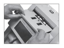
5 Remove feeder plate as shown at left.
