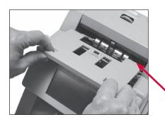
6 Replace the feeder plate. Insert the curved edge of the feeder plate first. Gently press down on the feeder plate until it snaps into position.
