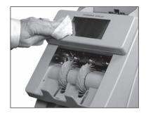
Clean remaining hard-plastic 16 exterior surfaces as necessary with a Simple Green Safety Towel.
