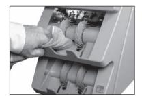
In pockets one and two, use a microfiber towel or vacuum to clean the stacker-sensor lens located between the two gray stacker wheels.
