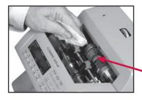
Use a Simple Green Safety Towel to clean all rubber sections of the large, black feed rollers. Rotate the rollers.
