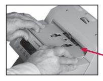
Replace feeder plate. Insert curved edge of feeder plate first. Gently press down on feeder plate until it snaps into position.
