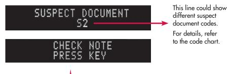
JetScan sensors have detected a possible counterfeit note. JetScan has stopped with this note as the top note in the bottom stacker. This note has not been included in the count.
