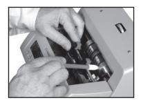
Use a Simple Green Safety Towel to remove dirt buildup from the upper and lower aluminum rollers. To reach all exposed surfaces, rotate the large, black feed rollers forward (direction of note flow). (See Helpful Hint.)
