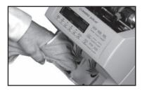
Use a microfiber towel or vacuum to remove any remaining dust in the bottom stacker.
