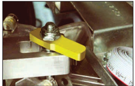
Incorrect: disk is not secured
