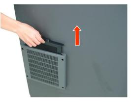
Cleaning method: Take the air filter out of its holder by pulling it upwards, wash it with water and dry completely, then restore the air filter.
