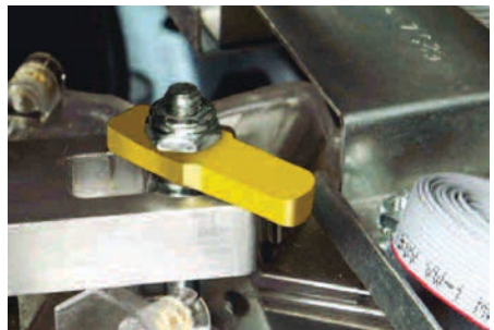
Incorrect: disk is not secured
