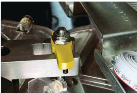
Correct: disk is secured
