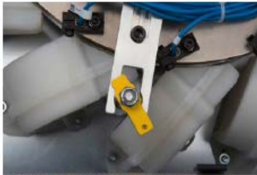
Incorrect: disk is not secured
