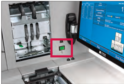
Master power switch ON
