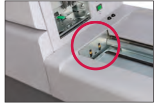
Rollers and start sensor in feeder
